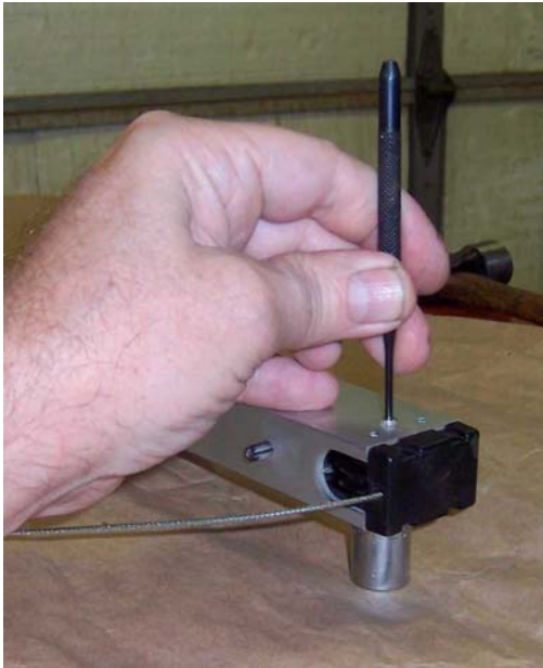
Punching out the top axle, closer supported by sockets
