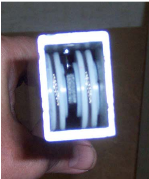
Rollers 1" from Bottom of closer extrusion
