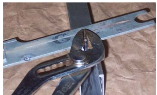
Pulling roll pin from extrusion
