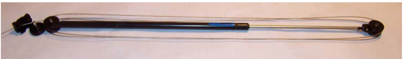
Internal parts of cable door closer- gas piston, 5 pulleys, top and bottom axles, cable
