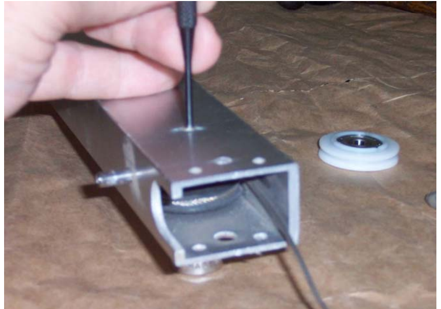
Punching out the lower pin, closer supported on sockets (output axle and pulley removed)
